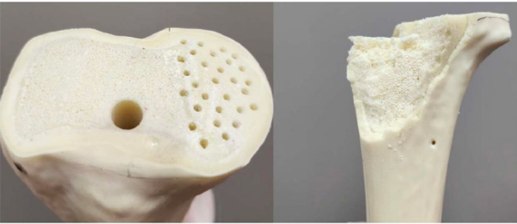
Fig. 2 (Abstract O41) Demonstrate the drilling pattern from group A synthetic sawbone study before (left) and after (Right) compression load to failure
