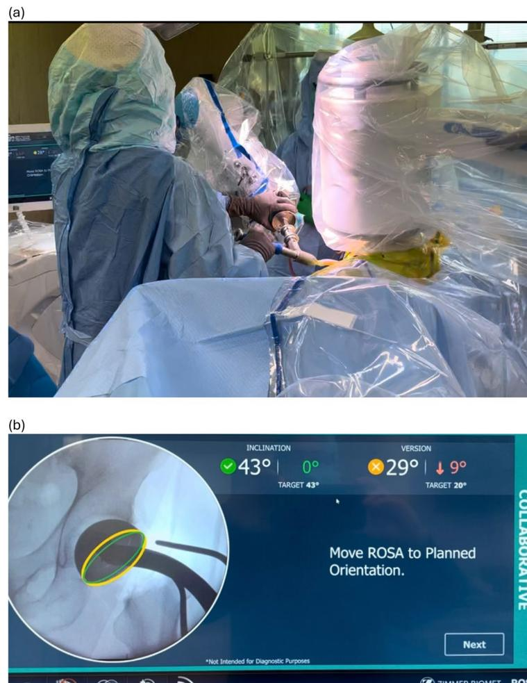
**Fig. 5** The ROSA robotic arm moves with surgeon collaboration (a) and haptic, visual and auditory feedback to the targeted inclination and version angles (b)
