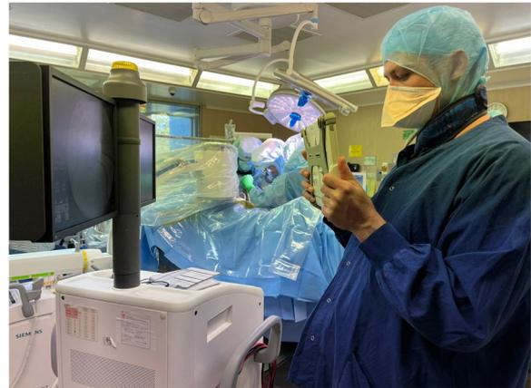
**Fig. 3** Images on the C-arm monitor are captured using the ROSA tablet by the ROSA support team and then transferred to the robotic system
